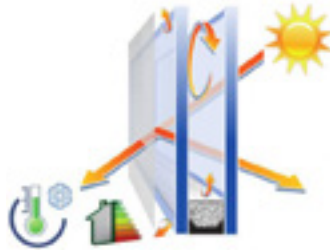
CLIMATE SCREEN MATERIAL 20.3% of heat is transmitted 79.7% of heat is reflected
