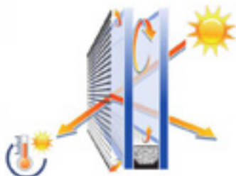
STANDARD SHADE FABRIC 75% of heat is transmitted 25% of heat is reflected
