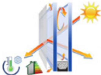
CLIMATE SCREEN MATERIAL 20.3% of heat is transmitted 79.7% of heat is reflected
